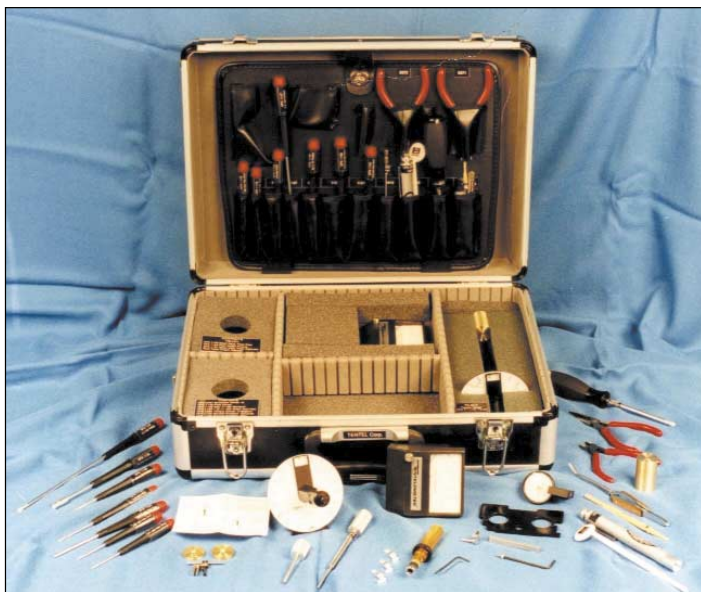
The Tentel DVCPRO kit includes specialized test and measurement tools and an array of standard hand tools. This keeps everything in one convenient case.
